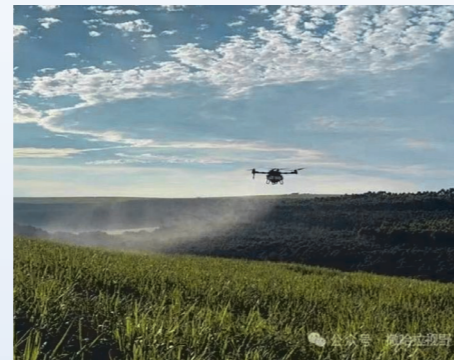
At Fountainhill Estate, KwaZulu Natal, South Africa, an XAG agricultural drone is spraying fungicide on a sugarcane field.
